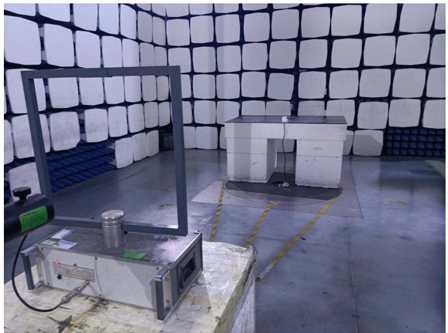
Radiation Emission Test Setup (Below 30MHz)
