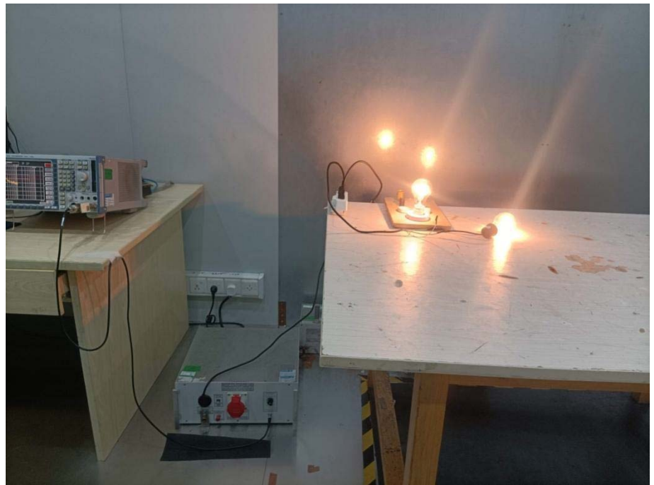
Conducted Emission Test Setup
