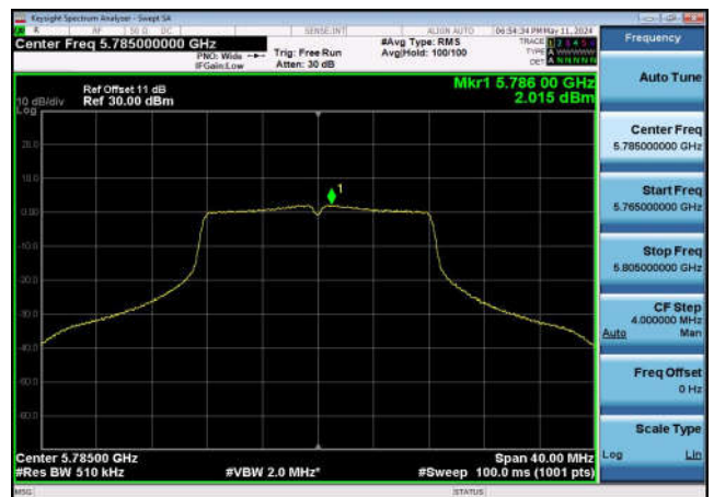
U-NII-3 Power spectral density-802.11 a(20MHz),5785MHz,Ant0
