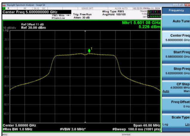
U-NII-2c Power spectral density-802.11 1a(20MHz),5600MHz,Ant0
