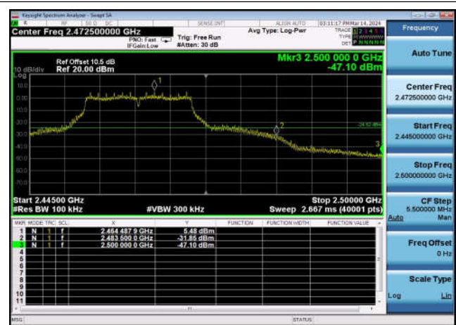
,Plot 2,Band Edge-802.11g,2462MHz ,Ant0
