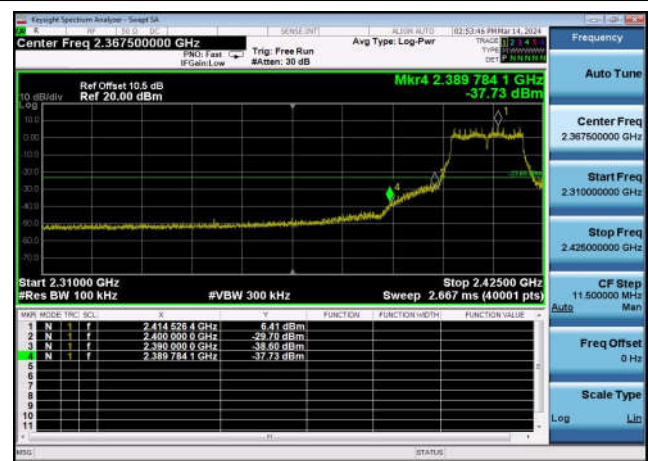
,Plot 2,Band Edge-802.11g,2462MHz ,Ant0
