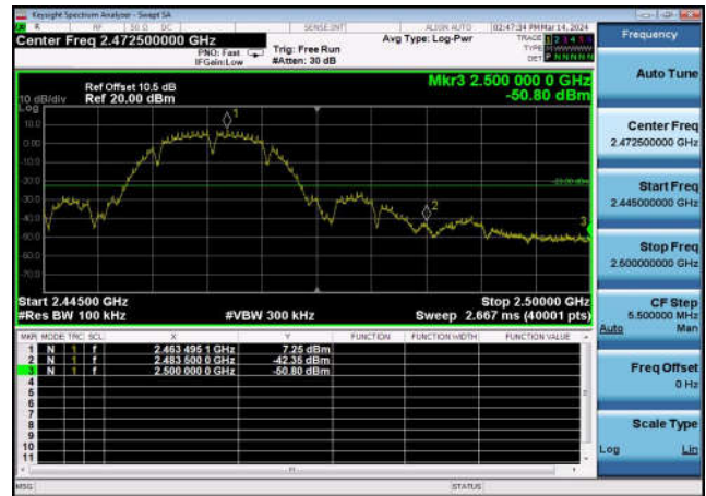
,Plot 2,Band Edge-802.11b,2462MHz ,Ant0
