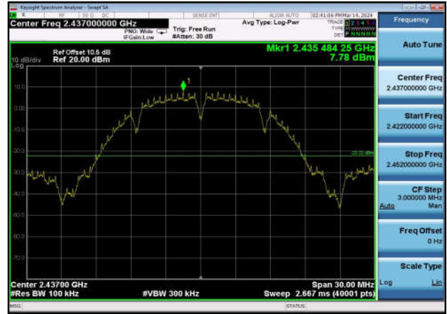
,Plot 2,Band Edge-802.11b,2412MHz ,Ant0
