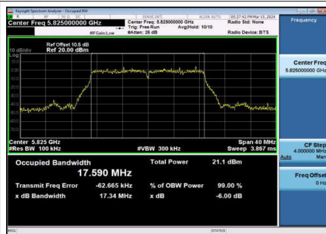
U-NII-3 6dB Bandwidth-802.11ax(20MHz) ,5785MHz,Ant1
