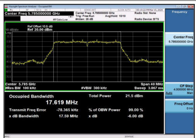
U-NII-3 6dB Bandwidth-802.11ax(20MHz) ,5745MHz,Ant1
