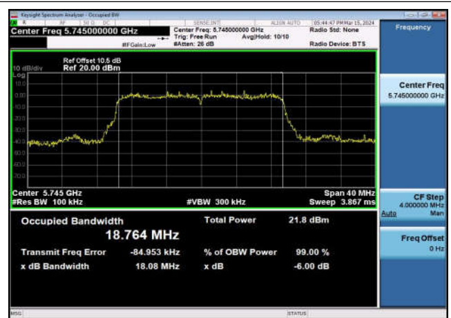
U-NII-3 6dB Bandwidth-802.11ax(20MHz) ,5825MHz,Ant1
