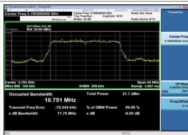
U-NII-3 6dB Bandwidth-802.11ax(20MHz) ,5785MHz,Ant1
