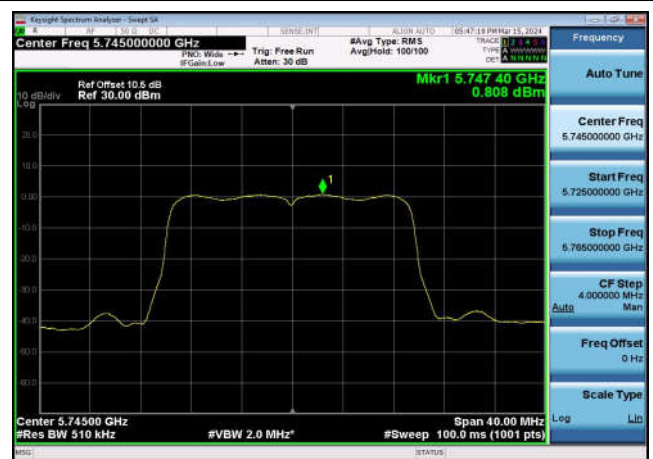
U-NII-3 Power spectral density-802.11 ax(20MHz),5825MHz,Ant1
