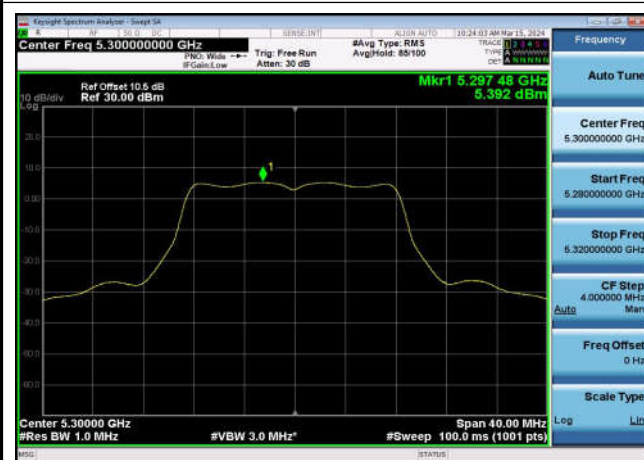
U-NII-2a Power spectral density-802.1 1a(20MHz),5300MHz,Ant1
