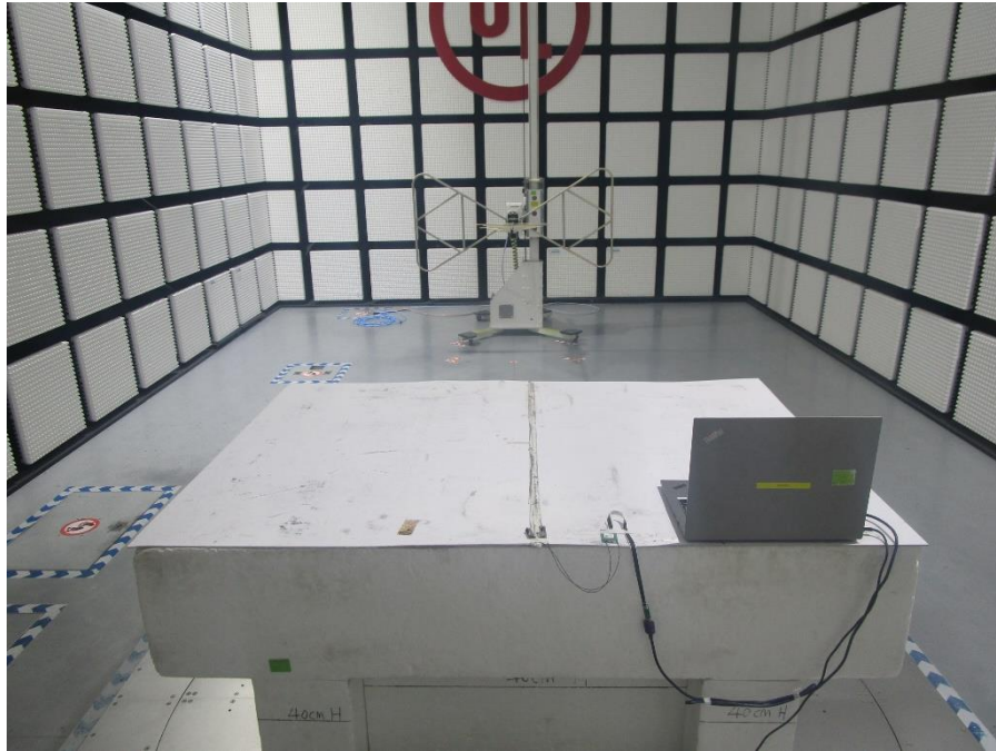
RADIATED RF MEASUREMENT SETUP (Below 30MHz)
