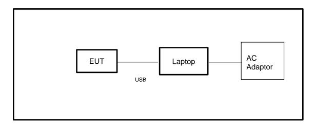
Note: AC Adaptor only use for AC POWER LINE CONDUCTED EMISSION test.
