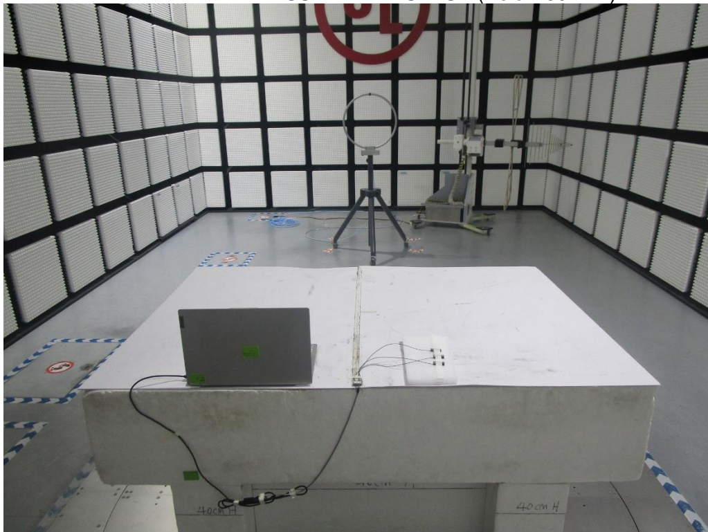
RADIATED RF MEASUREMENT SETUP (Below 30MHz)
