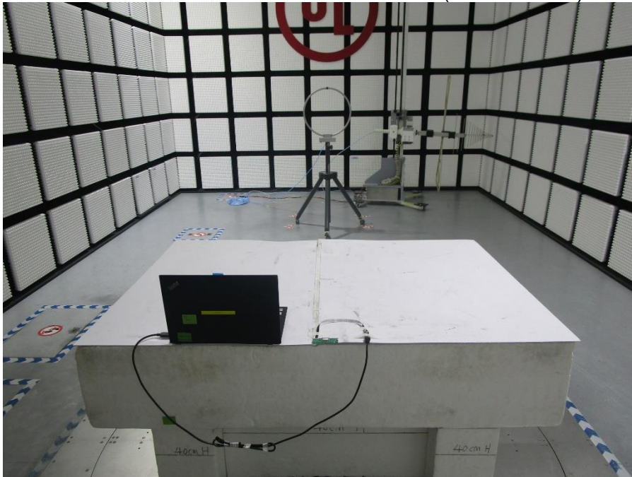
RADIATED RF MEASUREMENT SETUP (Below 30MHz)
