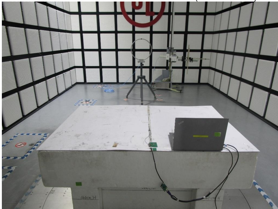
RADIATED RF MEASUREMENT SETUP (Below 30MHz)
