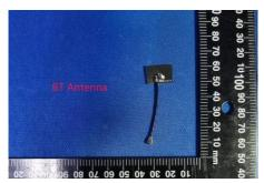
2.4G WIFI (2400-2500MHz) antenna gain is 0.52dBi and 0.48dBi. 5G WIFI (5000-6000MHz) antenna gain is 2.72dBi and 2.73dBi. BT (2400-2500MHz) antenna gain is 1.19dBi.
