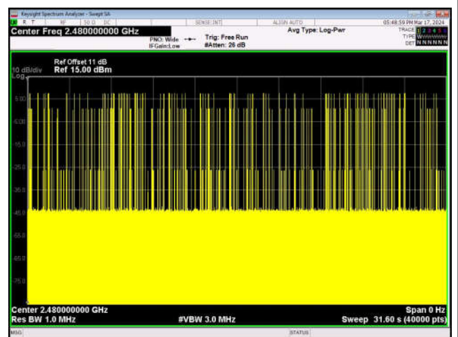
Number of Pulses in 31.6 seconds \pi/4 QPSK_2-DH5
