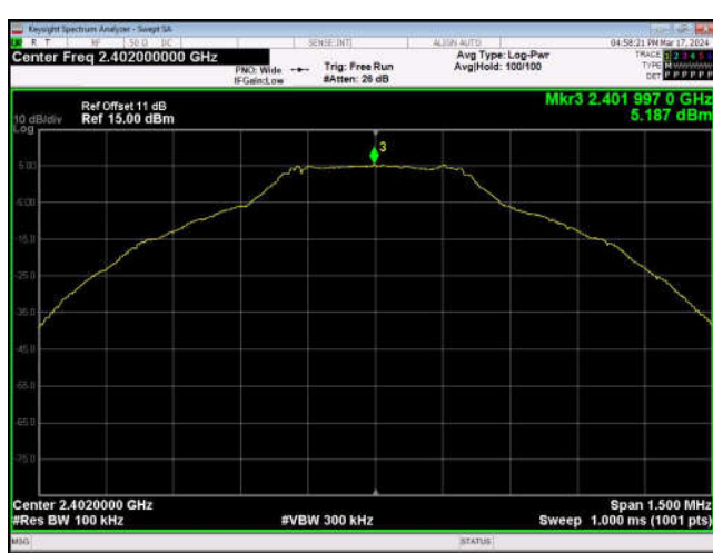
In-Band Reference Level GFSK_DH5_Channel 0
