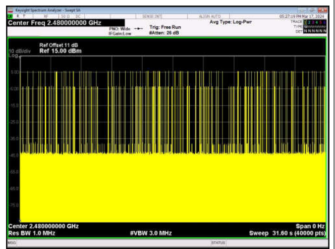
Number of Pulses in 31.6 seconds GFSK_DH5
