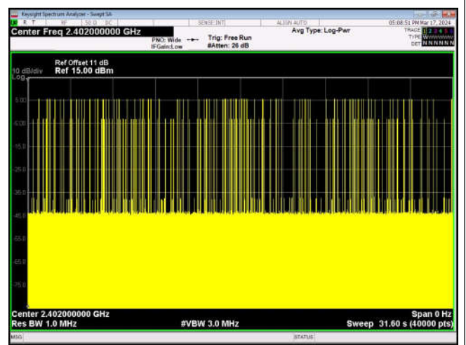
Number of Pulses in 31.6 seconds GFSK_DH5
