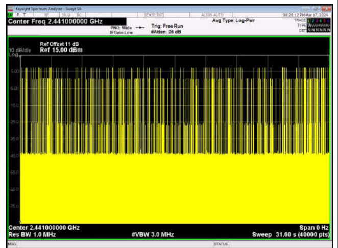
Number of Pulses in 31.6 seconds \pi/4 QPSK_2-DH5
