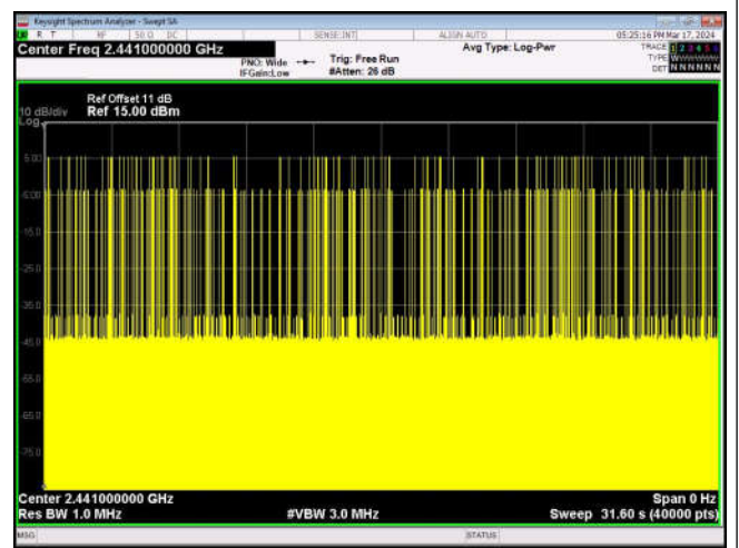
Number of Pulses in 31.6 seconds GFSK_DH5
