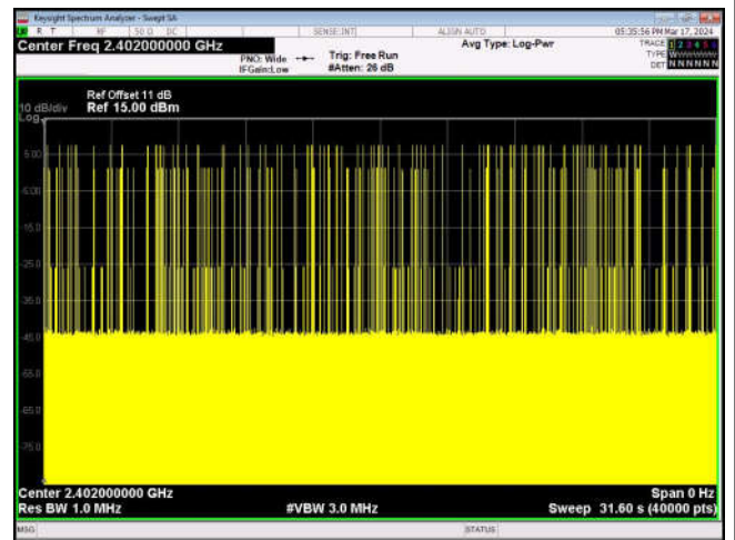
Number of Pulses in 31.6 seconds \pi/4 QPSK_2-DH5
