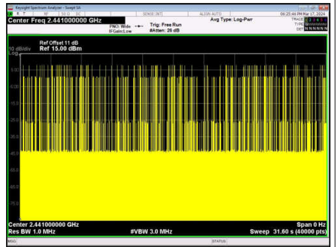
Number of Pulses in 31.6 seconds 8DPSK_3-DH5
