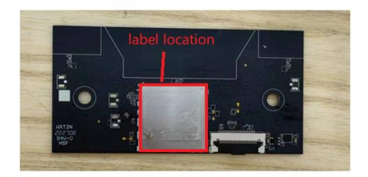
The label is attached to the surface of the shield with a permanent adhesive.
