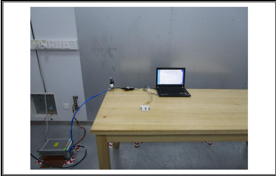
RADIATED RF MEASUREMENT SETUP (30MHz ~ 1 GHz)
