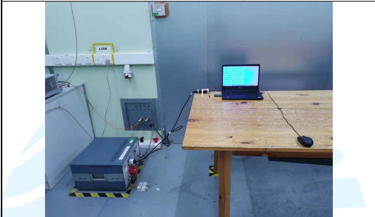
Conducted Emission Test Setup
