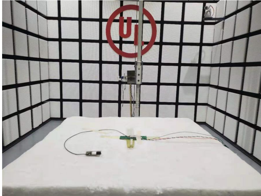
RADIATED RF MEASUREMENT SETUP (ABOVE 1 GHz) WIFI MEASUREMENT POSITION (X axis)
