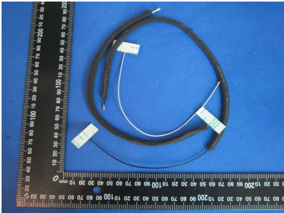
Photo 6 Appearance of Antenna
