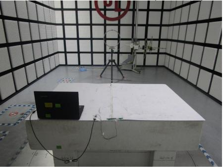
POWERLINE CONDUCTED EMISSIONS MEASUREMENT SETUP
