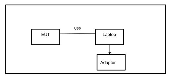
Note: Adapter only use for AC Power Line Conducted Emission testing.
