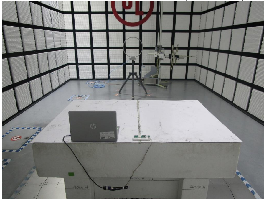
RADIATED RF MEASUREMENT SETUP (Below 30MHz)
