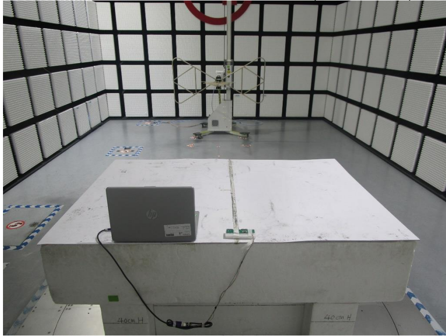
RADIATED RF MEASUREMENT SETUP (Below 30MHz)
