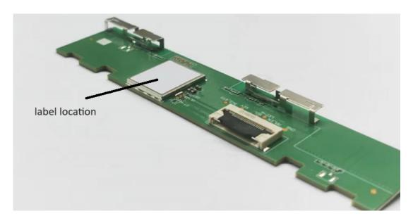
The label is attached to the surface of the shield with a permanent adhesive.
