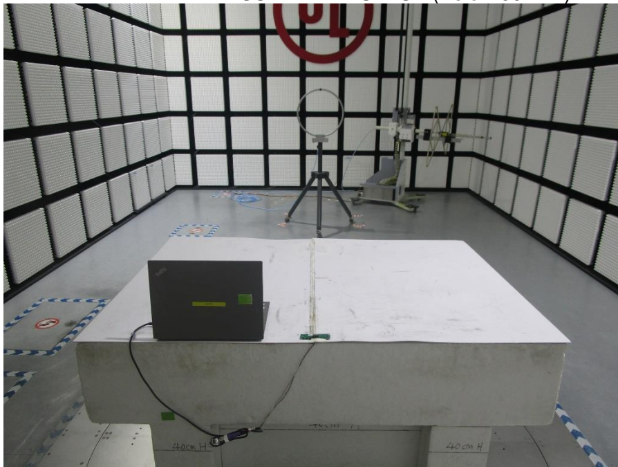
RADIATED RF MEASUREMENT SETUP (Below 30MHz)
