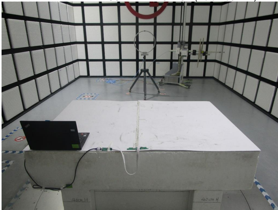
RADIATED RF MEASUREMENT SETUP (Below 30MHz)
