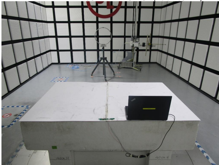
RADIATED RF MEASUREMENT SETUP (Below 30MHz)
