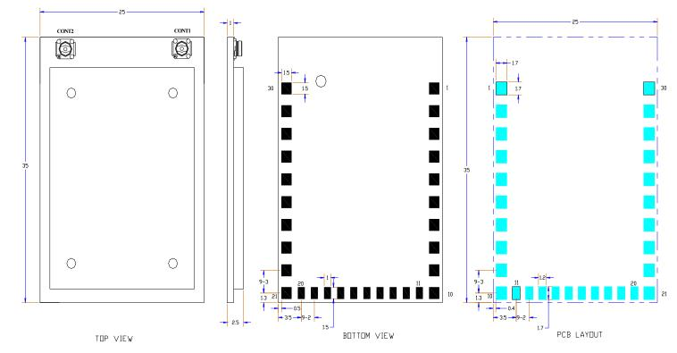
TOLERANCES ARE +/-0.3mm UNLESS OTHERWISE SPECIFIED \* UNITE :mm
