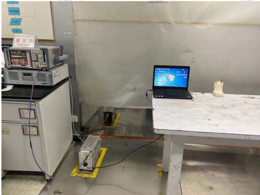
Conducted Emissions Test Setup-8
