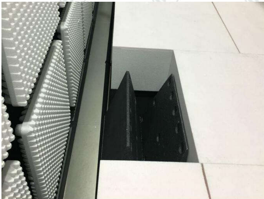
Radiated spurious emission Test Setup-6(Above 1GHz) There are absorbing materials under the ground.
