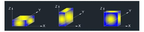
Note 1: For radiated test, EUT in each of three orthogonal axis emissions had been tested, but only the worst case (Y axis) data recorded in the report.
