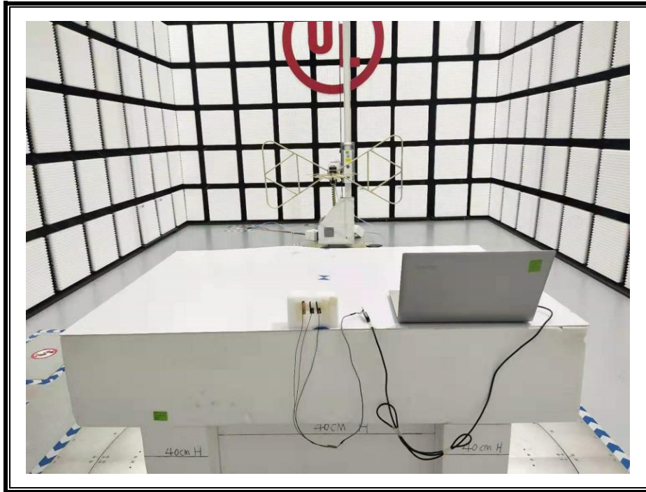
RADIATED RF MEASUREMENT SETUP (Below 30MHz)
