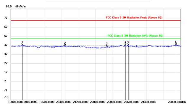
Reading Correct Result Limit Remark No. Frequency Margin (dBuV) (dB/m) (dBuV/m) (dBuV/m) (MHz) (dB) 18544.000 -4.4647.30 51.76 74.00 -26.70 peak 2 -5.00 20552.000 51.55 46.55 74.00 -27.45peak 3 22528.000 51.66 -5.79 45.87 74.00 -28.13 peak -4.96 4 23400.000 51.92 46.96 74.00 -27.04 peak 5 23536.000 51.96 -4.74 47.22 74.00 -26.78 peak 25784.000 49.23 -1.4947.74 74.00 -26.26 6 peak
