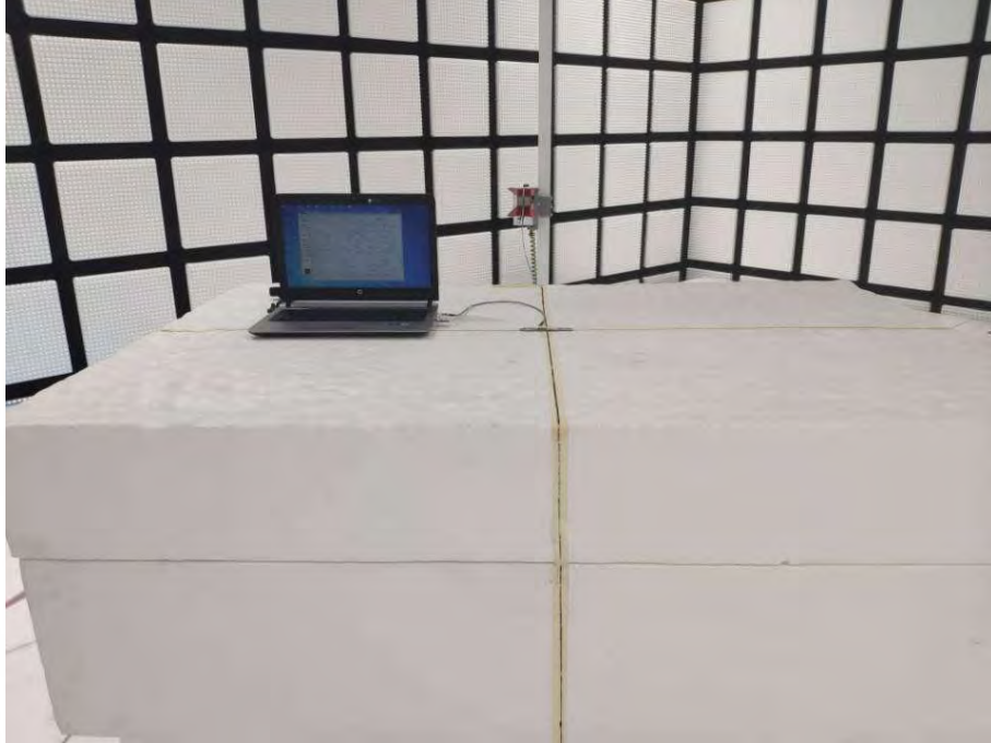
Radiated spurious emission Test Setup-2(Above 1GHz)
