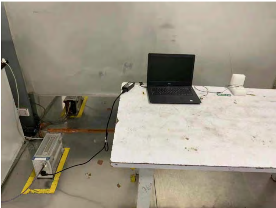
Conducted Emissions Test Setup
