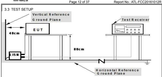
Note: 1. Support units were connected to second LISM. 2.Both of LISNs (AMN) are 80 cm from EUT and at least 80 from other units and other metal planes
