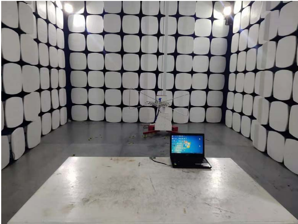
Test Setup Below 1GHz
