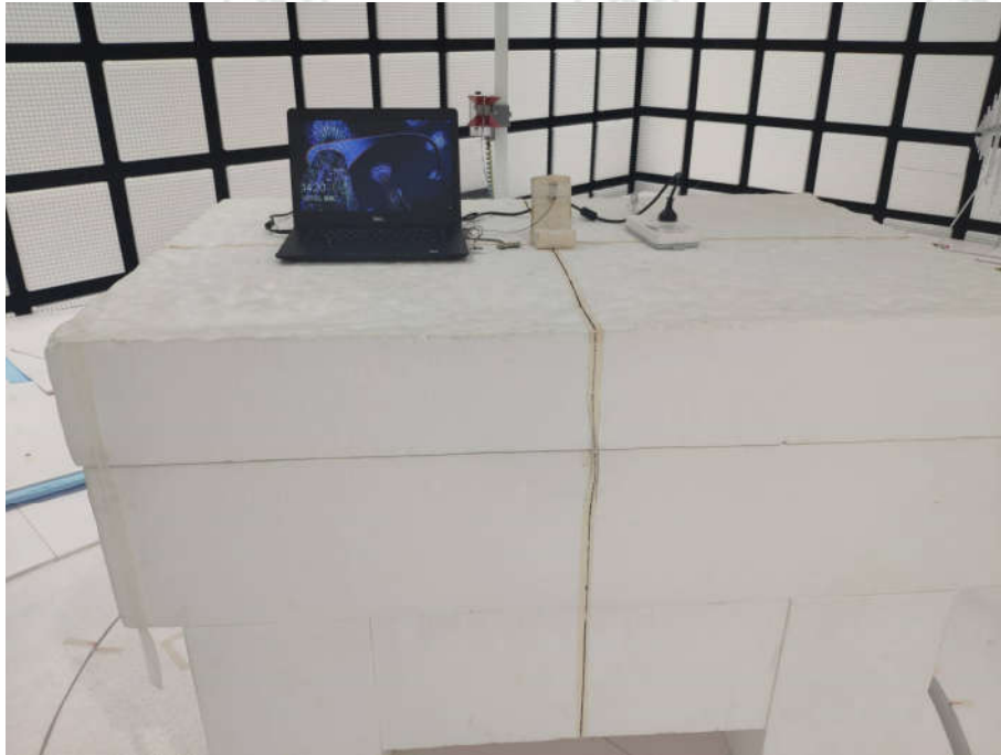
Radiated spurious emission Test Setup-3(Above 1GHz)
