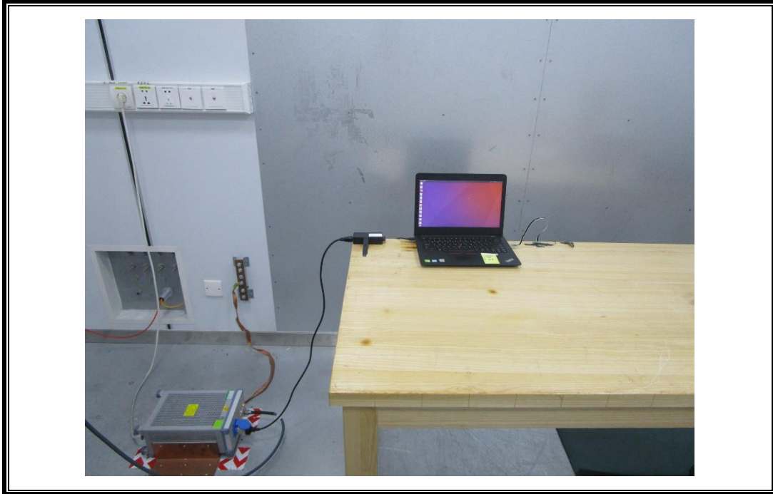
RADIATED RF MEASUREMENT SETUP (30MHz ~ 1 GHz)
