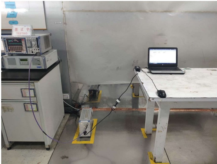
Conducted Emissions Test Setup
