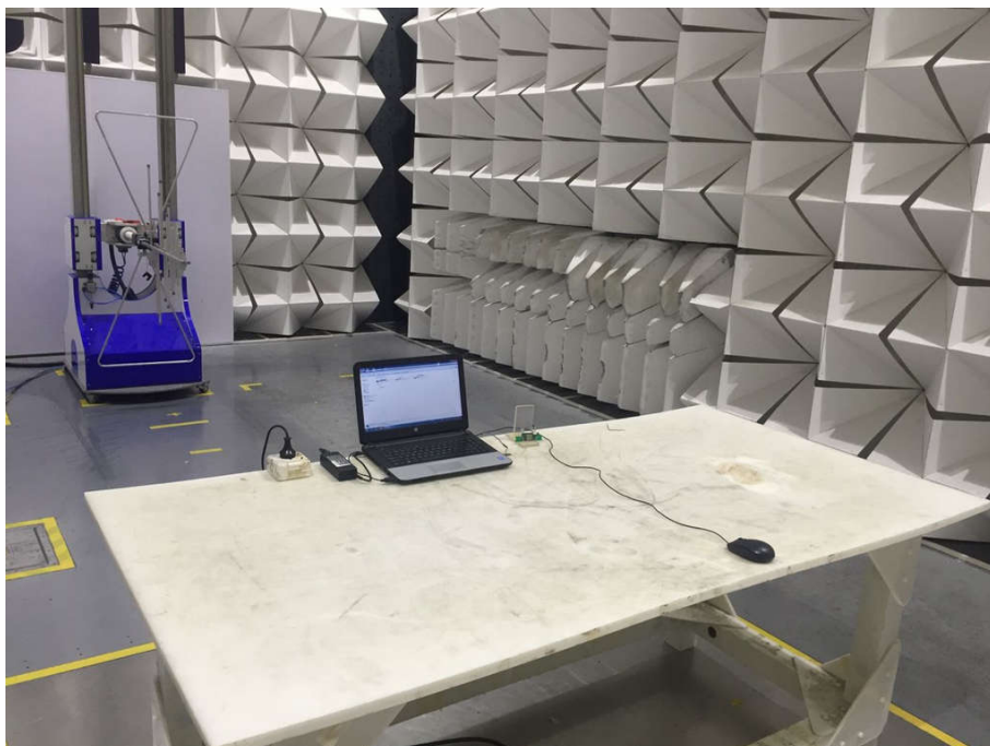
Radiated spurious emission Test Setup-2(30MHz-1GHz)
