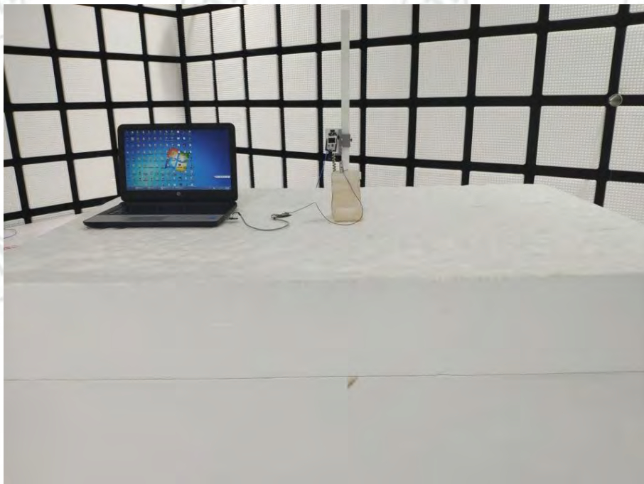
Radiated spurious emission Test Setup-4(Above 18GHz)
