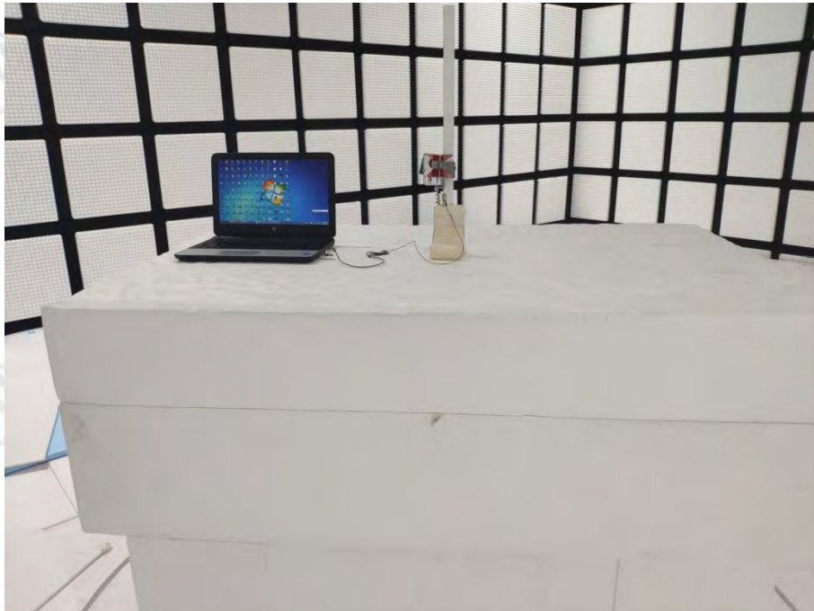
Radiated spurious emission Test Setup-3(1GHz-18GHz)
