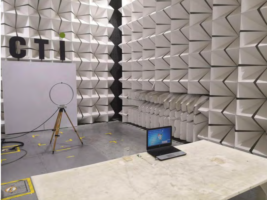
Radiated spurious emission Test Setup-1(Below 30MHz)
