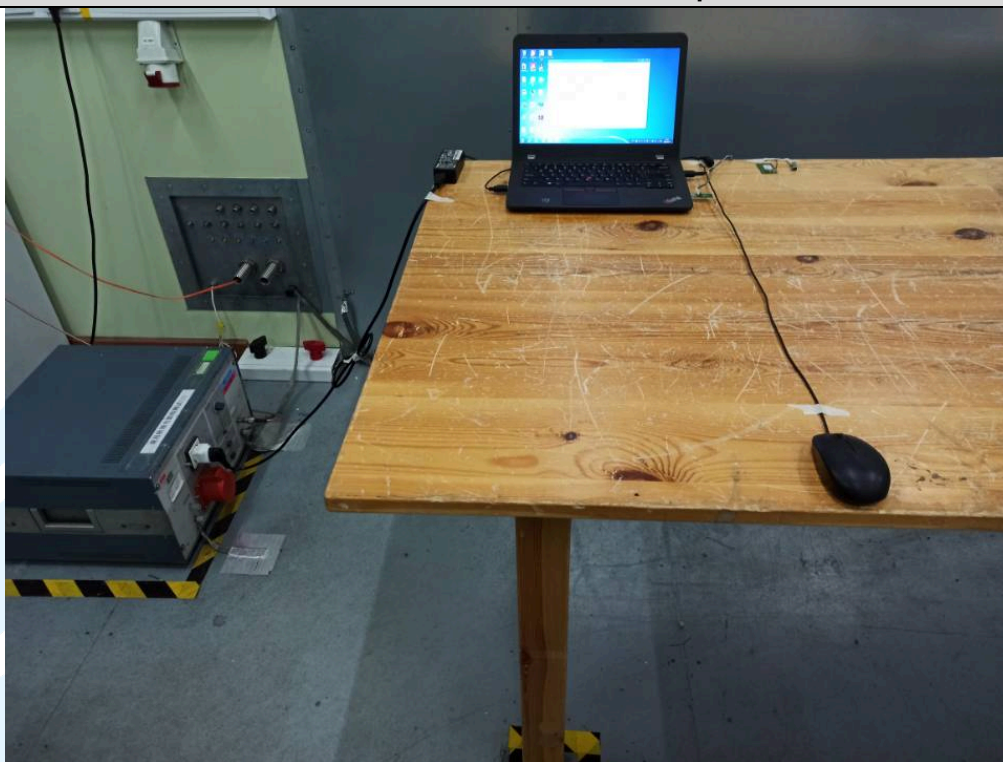
Conducted Emission Test Setup
