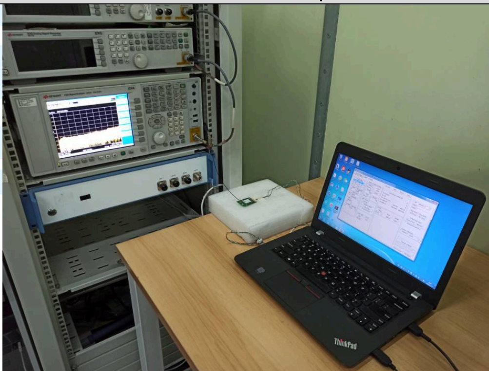
RF Conducted Test Setup
