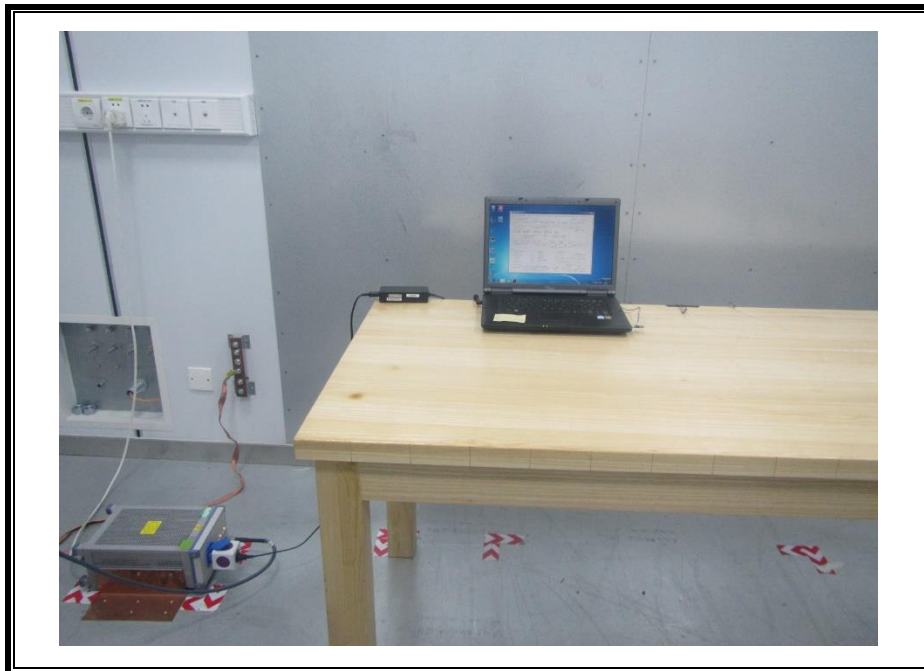
RADIATED RF MEASUREMENT SETUP (Below 30MHz)
