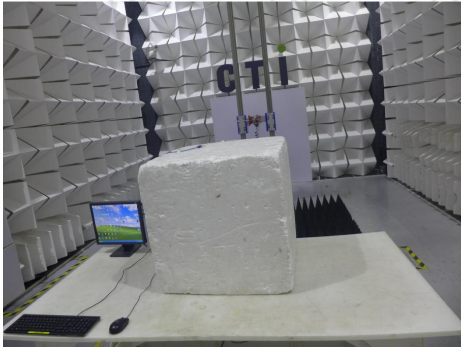
Radiated spurious emission Test Setup-3(Above 1GHz)
