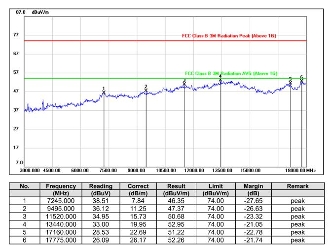
Note: 1. Measurement = Reading Level + Correct Factor.
