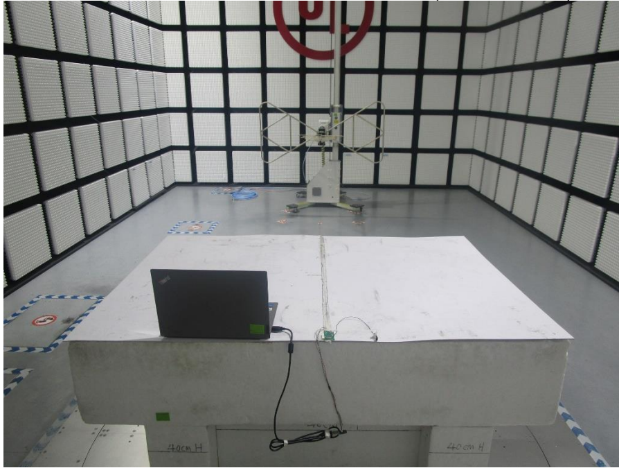
RADIATED RF MEASUREMENT SETUP (Below 30MHz)
