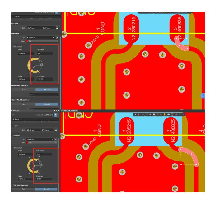
Note: 1. RF trace between module RF pinout to antenna width is 0.292mm. 2. RF trace between module and antenna impedance is 50ohm.
