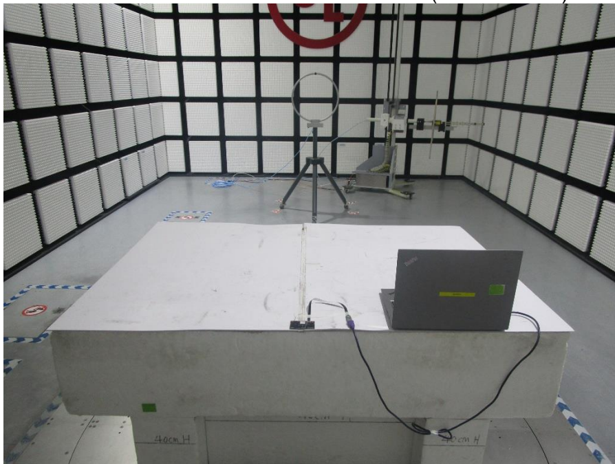
RADIATED RF MEASUREMENT SETUP (Below 30MHz)
