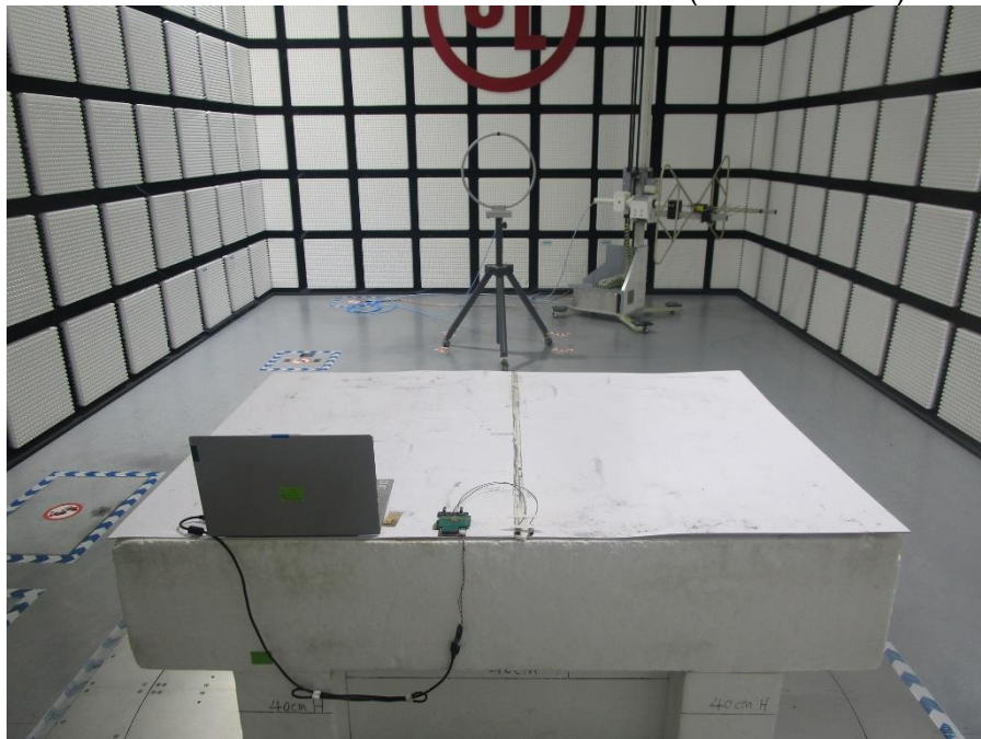
RADIATED RF MEASUREMENT SETUP (Below 30MHz)
