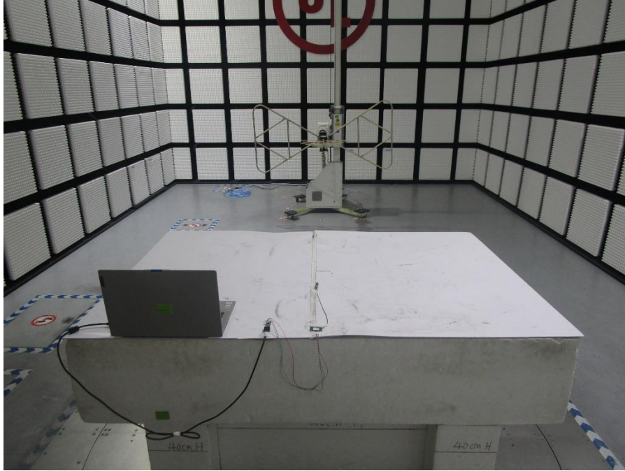
RADIATED RF MEASUREMENT SETUP (30MHz~1GHz)
