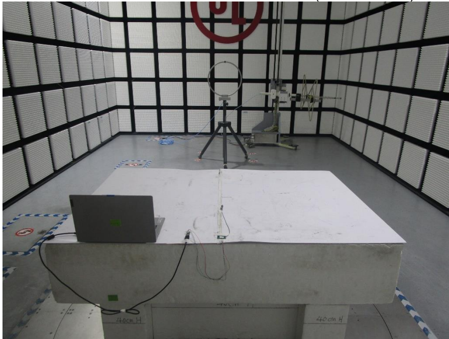
RADIATED RF MEASUREMENT SETUP (Below 30MHz)
