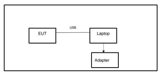
Note: Adapter only use for AC Power Line Conducted Emission testing.
