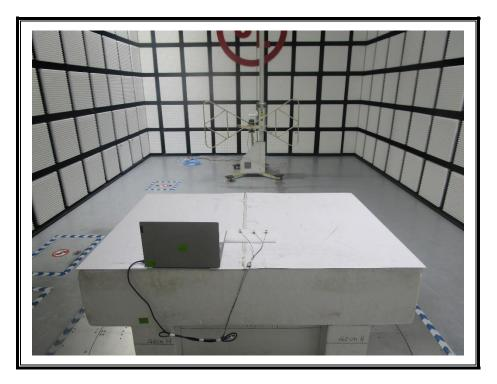
RADIATED RF MEASUREMENT SETUP (Below 30MHz)
