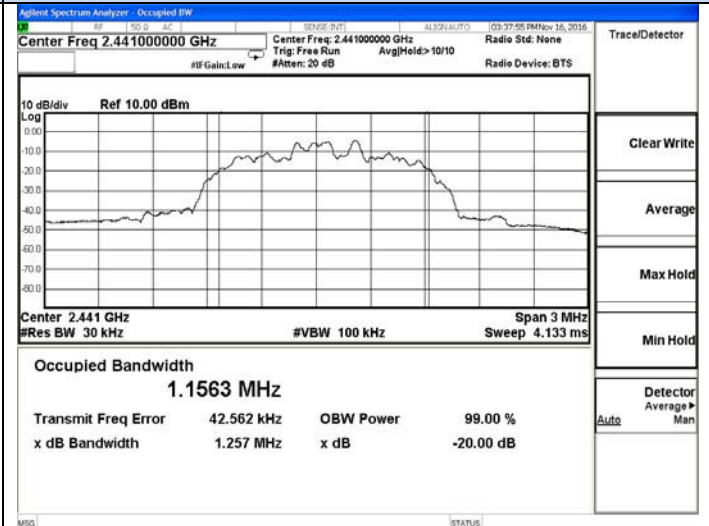
20dB Bandwidth \pi/4 -DQPSK-Middle channel
