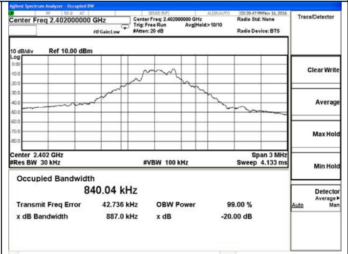
20dB Bandwidth GFSK-Low channel
