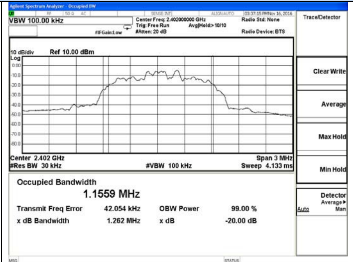
20dB Bandwidth \pi/4 -DQPSK-Low channel
