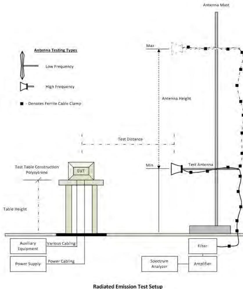
A full system calibration was performed on the test station and any resulting system losses (or gains) were taken into account in the production of all final measurement data.
