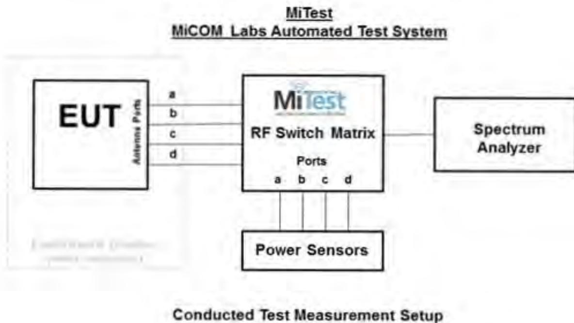
A full system calibration was performed on the test station and any resulting system losses (or gains) were taken into account in the production of all final measurement data.
